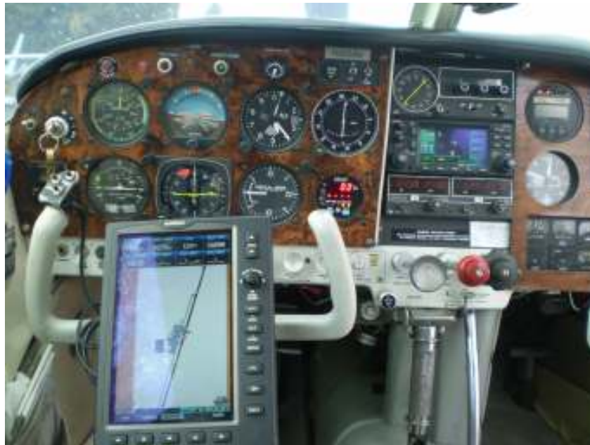
Dual Garmin GPSs (430W and 695), JPI Fuel totalizer on the lower right, STEC-30 Autopilot, King HSI.
